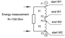
Observing the polarity a positive pulse is induced at press actuation and a negative pulse is induced at release actuation
